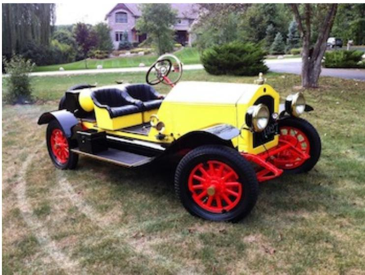
The Falcon Knight was a nameplate of the Willys-Overland complex. They were only made for two years and were intended to have a price point between the Whippet and the Willys. Stephen Plaster's Model 10 has a one-off Speedster body. The six-cylinder, sleeve valve engine combined with the lightweight body creates a high performance car of its day. The two individual seats and the monocle windshield add to the sporting feeling. *Pictured: Falcon Knight Model 10.*
